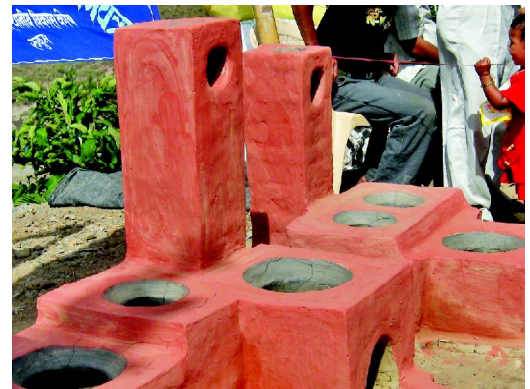
▲ Improved smokeless stove
